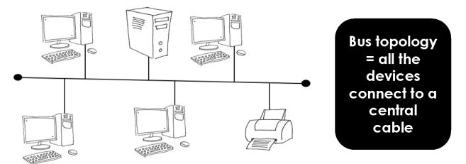
With a bus network, all the devices are connected to one central main cable called the "bus". At each end of the cable a terminator "•", which is fitted to stop signals reflecting down the bus. Each computer is responsible for sending message and listening to see if any ness on the network are meant for them.
